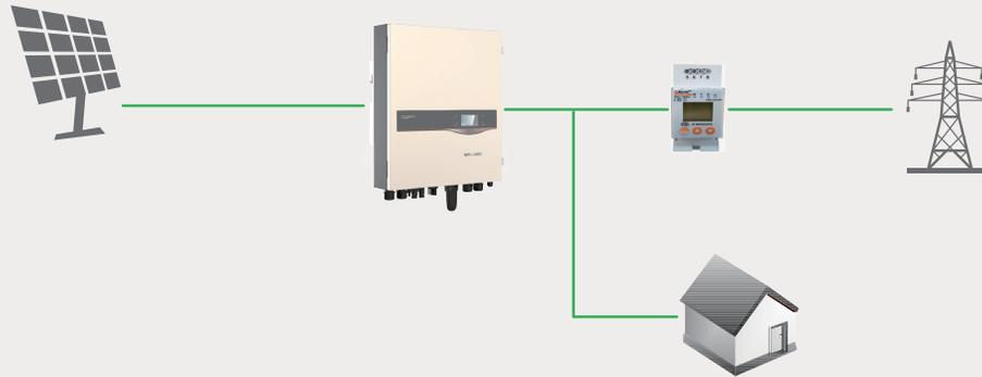
If the household loads and the PV generation curve are well matched, battery module may not be required, the SH5K hybrid inverter and meter could be used as a "Zero-export" system. In this system, the inverter output will be derated to ensure the feed-in power be zero when a feed-in power above zero is detected by the meter. The feed-in power threshold can be set ranging from 0 to 5000 W. If the threshold value is set to 5000 W, all excessive power will be exported.
